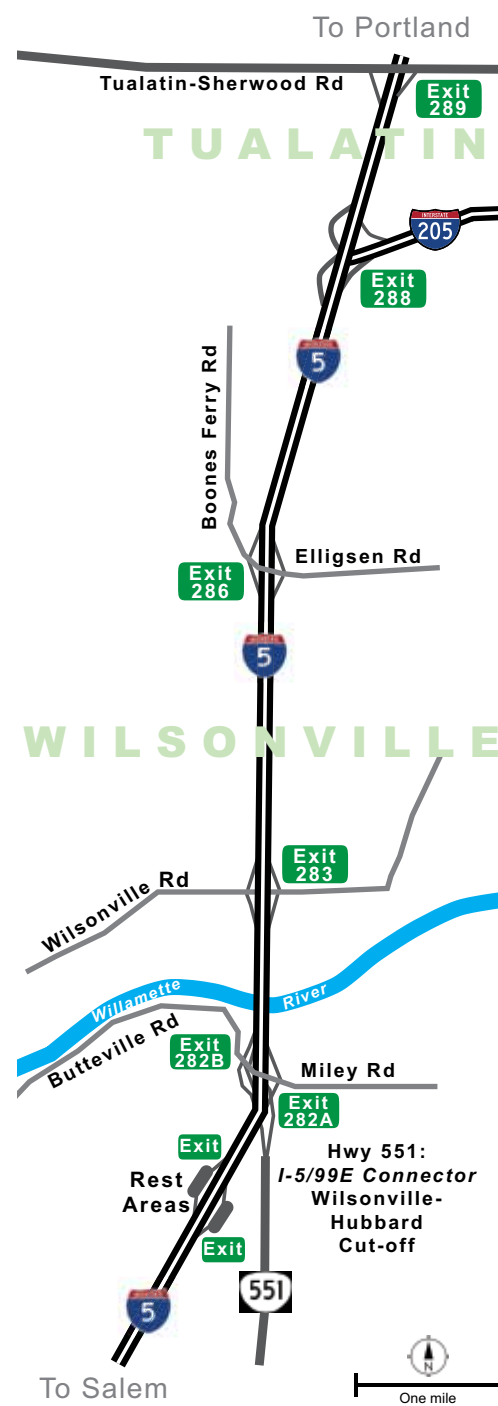
Map illustrating I-5 exits in the Wilsonville area. Each interchange on/off ramp introduces automobile weaving lane-changes that are a major contributor to traffic congestion and highway incidents.
