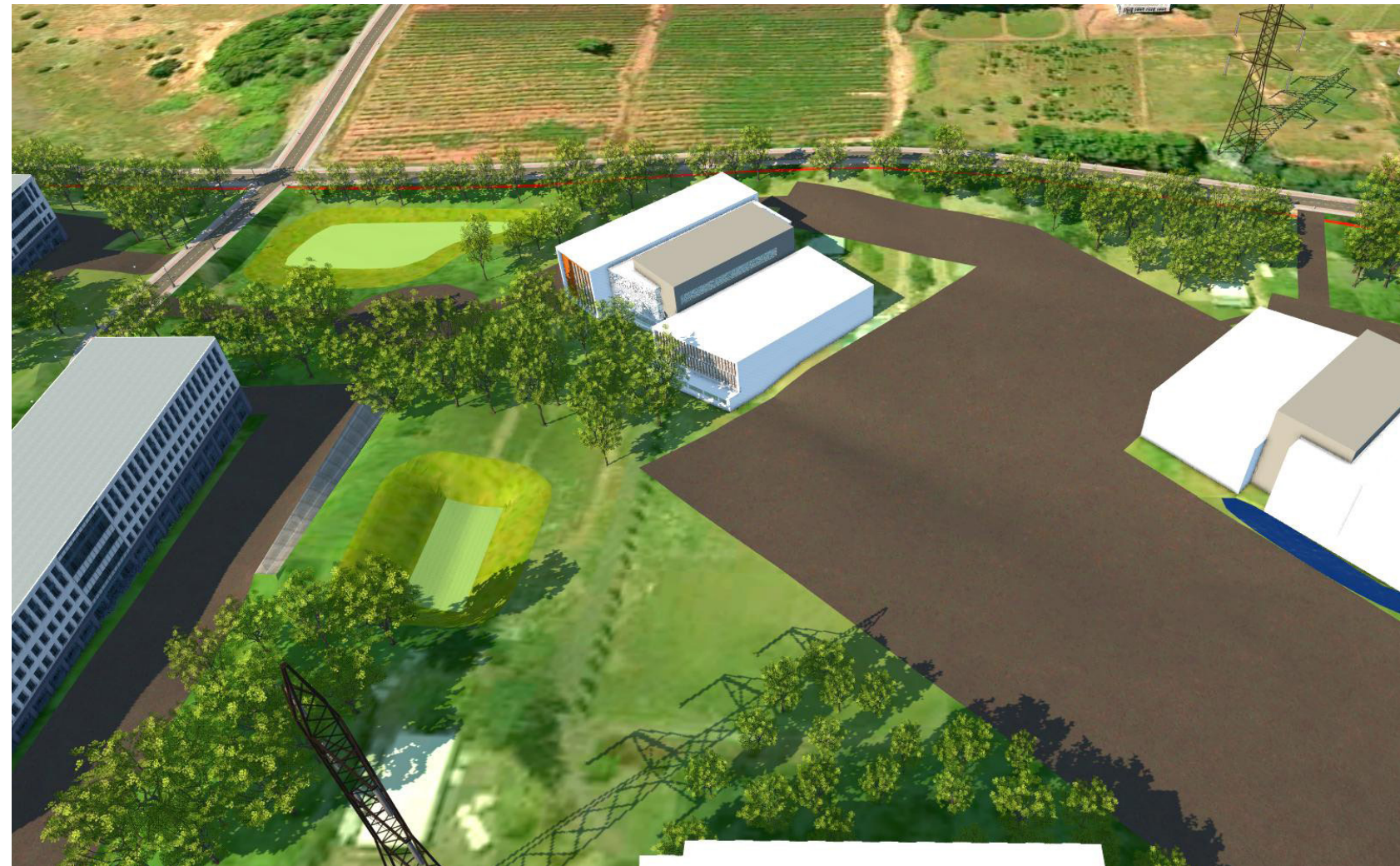
Scheme B Stormwater Pond
