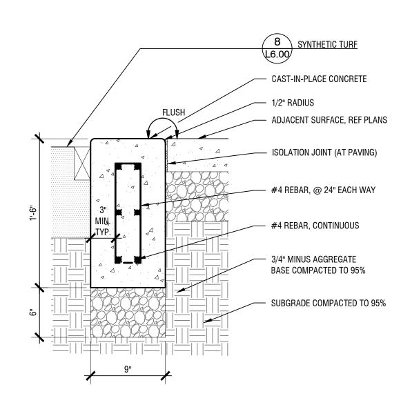
$\uparrow$  CONCRETE HEADER, TYPE 1 - SECTION **1** SCALE: 1 1/2"= 1'-0"
