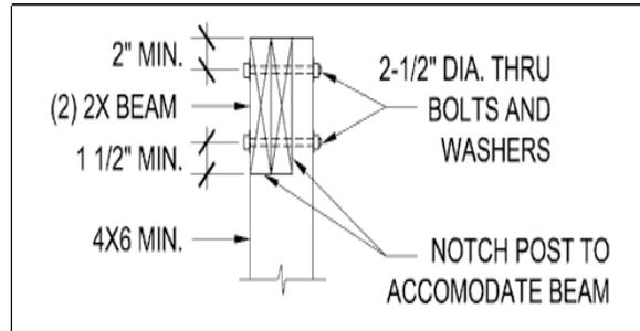
Figure 21 - Post-to-Beam Requirements
