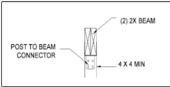
Figure 20 - Post-to-Beam Requirements
