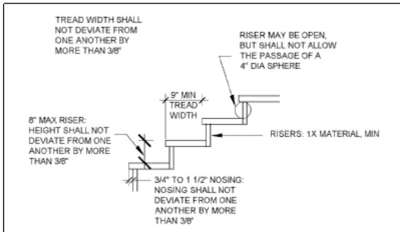
Figure 30 - Tread and Riser Detail
