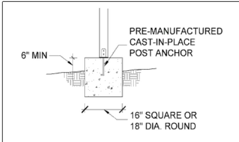
Figure 22 - Typical Footing Detail
