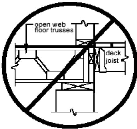
Figure 8: No Attachment To Open Web Trusses
