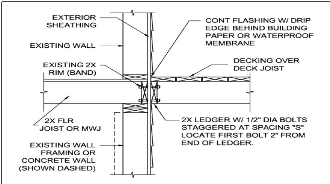
Figure 6 – Attachment of Ledger Board to Band Board with Bolts.
