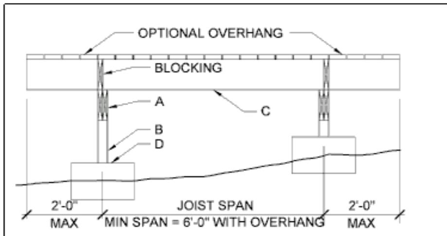
Figure 2 - Joist Span - Free-Standing Deck
