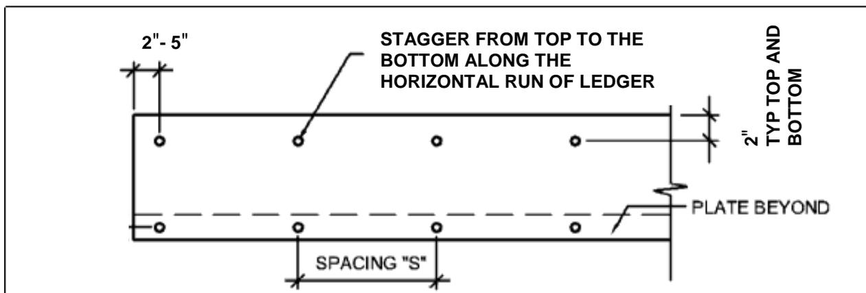
Figure 11 - Ledger Board Fastener Spacing and Clearances
