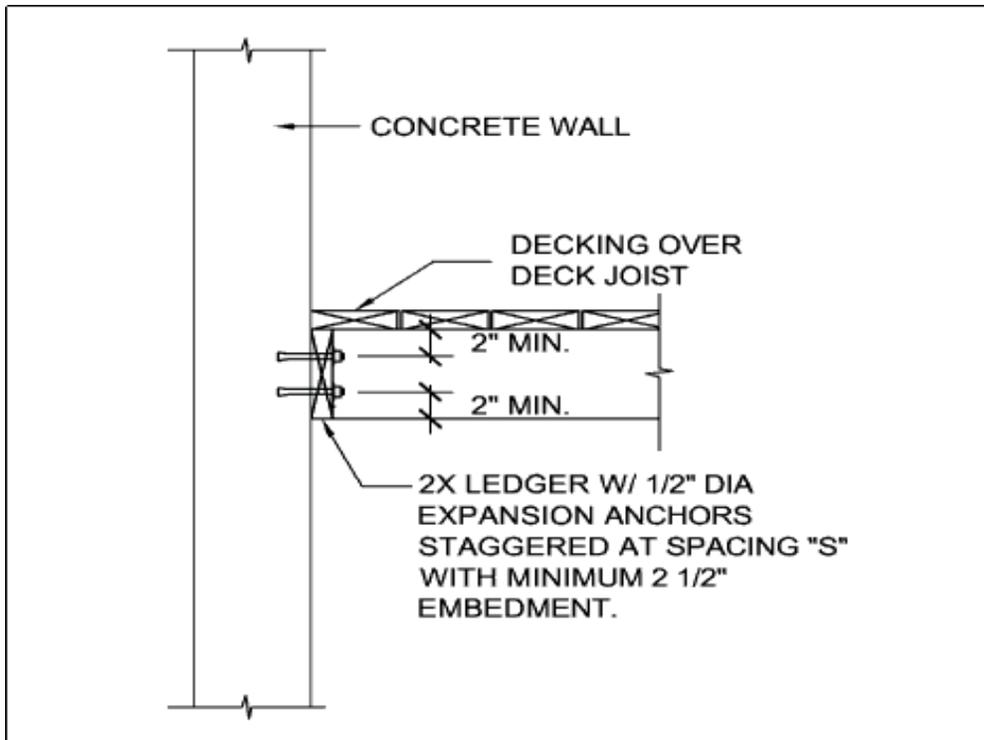
Figure 7 – Attachment of Ledger Board to Concrete Wall.
